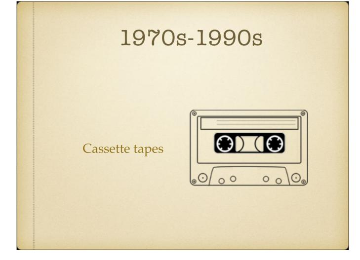
The compact cassette is a magnetic tape recording format for audio recording and playback. Cassettes consist of two miniature spools, between which a magnetically coated plastic tape is passed and wound. These spools and their attendant parts are held inside a protective plastic shell. Cassettes held typically 30 or 45 minutes of audio per side.
